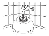
Rinse with hot water. Clean the water tank with acetic cleaning agent as required, then thoroughly rinse with fresh water
